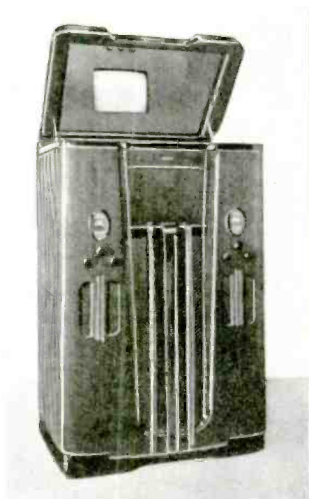
Front view of the Philco television receiver with "image" and "sound" tuning dials at right and left of cabinet.
